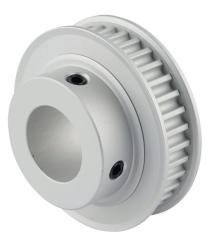
Sung-Il Machinery timing pulley, aluminum, 5mm 5M pitch, 36 tooth, 2.256in pitch diameter, 7/8in bore, hub with flanges. For use with 9mm wide belt.
