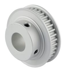
Sung-Il Machinery timing pulley, aluminum, 5mm 5M pitch, 36 tooth, 2.256in pitch diameter, 3/4in bore, hub with flanges. For use with 9mm wide belt.
