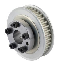
Sung-Il Machinery timing pulley, aluminum, 5mm 5M pitch, 36 tooth, 2.256in pitch diameter, 5/8in bore, no hub with flanges. For use with 9mm wide belt. QD bushing included.
