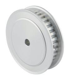
Sung-Il Machinery timing pulley, aluminum, 1/5in XL pitch, 32 tooth, 2.037in pitch diameter, 1/4in bore, no hub with flanges. For use with 3/8in wide belt.
