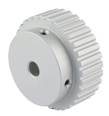
Sung-II Machinery timing pulley, aluminum, 1/5in XL pitch, 32 tooth, 2.037in pitch diameter, 5/16in bore, hub without flanges. For use with 3/8in wide belt.
