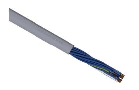
LUTZE Silflex flexible control cable, unshielded, 19 conductors (includes ground), 18 AWG, bare copper, PVC/Nylon conductor insulation material, blue with white numbers and green/yellow ground, #2 conductor is white/blue, PVC jacket, gray, cut to length.
