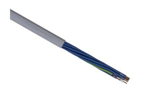
LUTZE Silflex flexible control cable, unshielded, 12 conductors (includes ground), 18 AWG, bare copper, PVC/Nylon conductor insulation material, blue with white numbers and green/yellow ground, #2 conductor is white/blue, PVC jacket, gray, cut to length.
