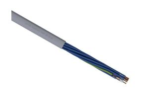
LUTZE Silflex flexible control cable, unshielded, 12 conductors (includes ground), 18 AWG, bare copper, PVC/Nylon conductor insulation material, blue with white numbers and green/yellow ground, #2 conductor is white/blue, PVC jacket, gray, cut to length.
