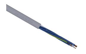
LUTZE Silflex flexible control cable, unshielded, 7 conductors (includes ground), 18 AWG, bare copper, PVC/Nylon conductor insulation material, blue with white numbers and green/yellow ground, #2 conductor is white/blue, PVC jacket, gray, cut to length.
