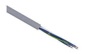
LUTZE Silflex flexible control cable, unshielded, 5 conductors (includes ground), 18 AWG, bare copper, PVC/Nylon conductor insulation material, blue with white numbers and green/yellow ground, #2 conductor is white/blue, PVC jacket, gray, cut to length.
