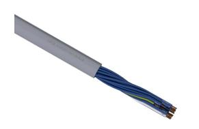
LUTZE Silflex flexible control cable, unshielded, 19 conductors (includes ground), 16 AWG, bare copper, PVC/Nylon conductor insulation material, blue with white numbers and green/yellow ground, #2 conductor is white/blue, PVC jacket, gray, cut to length.
