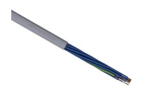
LUTZE Silflex flexible control cable, unshielded, 12 conductors (includes ground), 16 AWG, bare copper, PVC/Nylon conductor insulation material, blue with white numbers and green/yellow ground, #2 conductor is white/blue, PVC jacket, gray, cut to length.
