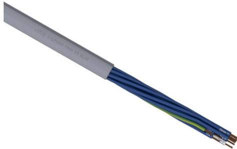
LUTZE Silflex flexible control cable, unshielded, 12 conductors (includes ground), 16 AWG, bare copper, PVC/Nylon conductor insulation material, blue with white numbers and green/yellow ground, #2 conductor is white/blue, PVC jacket, gray, cut to length.
