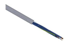
LUTZE Silflex flexible control cable, unshielded, 7 conductors (includes ground), 16 AWG, bare copper, PVC/Nylon conductor insulation material, blue with white numbers and green/yellow ground, #2 conductor is white/blue, PVC jacket, gray, cut to length.
