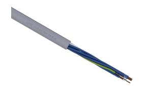
LUTZE Silflex flexible control cable, unshielded, 7 conductors (includes ground), 16 AWG, bare copper, PVC/Nylon conductor insulation material, blue with white numbers and green/yellow ground, #2 conductor is white/blue, PVC jacket, gray, cut to length.
