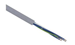
LUTZE Silflex flexible control cable, unshielded, 5 conductors (includes ground), 16 AWG, bare copper, PVC/Nylon conductor insulation material, blue with white numbers and green/yellow ground, #2 conductor is white/blue, PVC jacket, gray, cut to length.
