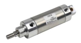
NITRA pneumatic cylinder, non-repairable, 2in bore, 5/8in rod diameter, 14in stroke, double acting, double end mount.
