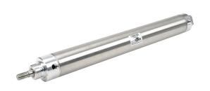
NITRA pneumatic cylinder, non-repairable, 2in bore, 5/8in rod diameter, 14in stroke, double acting, magnetic piston, double end mount
