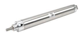
NITRA pneumatic cylinder, non-repairable, 2in bore, 5/8in rod diameter, 12in stroke, double acting, double end mount.
