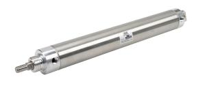
NITRA pneumatic cylinder, non-repairable, 2in bore, 5/8in rod diameter, 12in stroke, double acting, magnetic piston, double end mount.
