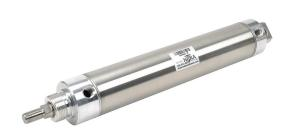
NITRA pneumatic cylinder, non-repairable, 2in bore, 5/8in rod diameter, 8in stroke, double acting, magnetic piston, double end mount.
