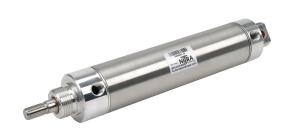
NITRA pneumatic cylinder, non-repairable, 2in bore, 5/8in rod diameter, 6in stroke, double acting, magnetic piston, double end mount.
