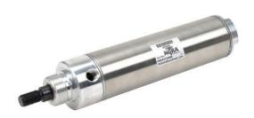
NITRA pneumatic cylinder, non-repairable, 2in bore, 5/8in rod diameter, 5in stroke, double acting, front nose mount.
