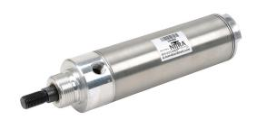
NITRA pneumatic cylinder, non-repairable, 2in bore, 5/8in rod diameter, 4in stroke, double acting, front nose mount.
