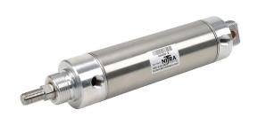
NITRA pneumatic cylinder, non-repairable, 2in bore, 5/8in rod diameter, 4in stroke, double acting, magnetic piston, double end mount
