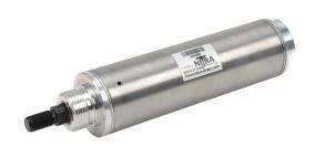
NITRA pneumatic cylinder, non-repairable, 2in bore, 5/8in rod diameter, 3in stroke, single acting, front nose mount.
