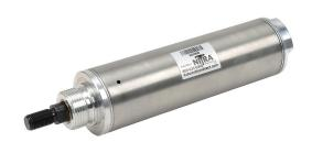
NITRA pneumatic cylinder, non-repairable, 2in bore, 5/8in rod diameter, 3in stroke, single acting, front nose mount.
