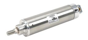
NITRA pneumatic cylinder, non-repairable, 2in bore, 5/8in rod diameter, 3in stroke, single acting, double end mount.
