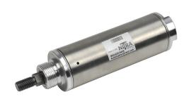
NITRA pneumatic cylinder, non-repairable, 2in bore, 5/8in rod diameter, 2in stroke, single acting, front nose mount.
