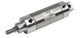
NITRA pneumatic cylinder, non-repairable, 2in bore, 5/8in rod diameter, 2in stroke, double acting, double end mount.
