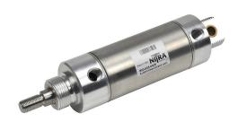
NITRA pneumatic cylinder, non-repairable, 2in bore, 5/8in rod diameter, 2in stroke, double acting, magnetic piston, double end mount.
