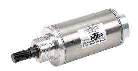
NITRA pneumatic cylinder, non-repairable, 2in bore, 5/8in rod diameter, 1in stroke, single acting, front nose mount.
