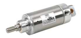
NITRA pneumatic cylinder, non-repairable, 2in bore, 5/8in rod diameter, 1in stroke, single acting, double end mount.
