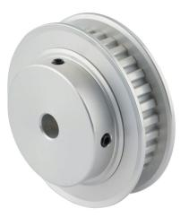
Sung-Il Machinery timing pulley, aluminum, 1/5in XL pitch, 32 tooth, 2.037in pitch diameter, 5/16in bore, hub with flanges. For use with 3/8in wide belt.
