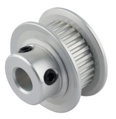
Sung-II Machinery timing pulley, aluminum, 0.08in MXL pitch, 32 tooth, 0.815in pitch diameter, 1/4in bore, hub with flanges. For use with 1/4in wide belt.
