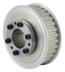
Sung-Il Machinery timing pulley, aluminum, 3/8in L pitch, 32 tooth, 3.82in pitch diameter, 1-1/4in bore, no hub with flanges. For use with 1in wide belt. QD bushing included.
