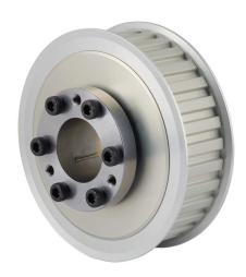
Sung-Il Machinery timing pulley, aluminum, 3/8in L pitch, 32 tooth, 3.82in pitch diameter, 1-1/8in bore, no hub with flanges. For use with 1in wide belt. QD bushing included.
