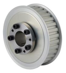
Sung-Il Machinery timing pulley, aluminum, 3/8in L pitch, 32 tooth, 3.82in pitch diameter, 1in bore, no hub with flanges. For use with 1in wide belt. QD bushing included.
