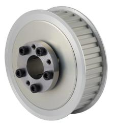
Sung-Il Machinery timing pulley, aluminum, 3/8in L pitch, 32 tooth, 3.82in pitch diameter, 7/8in bore, no hub with flanges. For use with 1in wide belt. QD bushing included.
