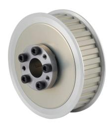
Sung-II Machinery timing pulley, aluminum, 3/8in L pitch, 32 tooth, 3.82in pitch diameter, 3/4in bore, no hub with flanges. For use with 1in wide belt. QD bushing included.
