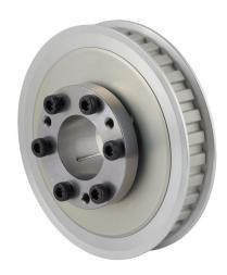
Sung-II Machinery timing pulley, aluminum, 3/8in L pitch, 32 tooth, 3.82in pitch diameter, 1-1/8in bore, no hub with flanges. For use with 1/2in wide belt. QD bushing included.
