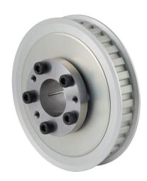
Sung-II Machinery timing pulley, aluminum, 3/8in L pitch, 32 tooth, 3.82in pitch diameter, 1in bore, no hub with flanges. For use with 1/2in wide belt. QD bushing included.
