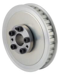
Sung-Il Machinery timing pulley, aluminum, 3/8in L pitch, 32 tooth, 3.82in pitch diameter, 3/4in bore, no hub with flanges. For use with 1/2in wide belt. QD bushing included.
