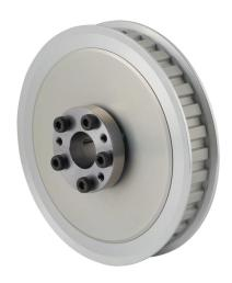
Sung-II Machinery timing pulley, aluminum, 3/8in L pitch, 32 tooth, 3.82in pitch diameter, 5/8in bore, no hub with flanges. For use with 1/2in wide belt. QD bushing included.
