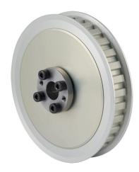
Sung-Il Machinery timing pulley, aluminum, 3/8in L pitch, 32 tooth, 3.82in pitch diameter, 1/2in bore, no hub with flanges. For use with 1/2in wide belt. QD bushing included.
