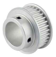
Sung-Il Machinery timing pulley, aluminum, 5mm 5M pitch, 32 tooth, 2.005in pitch diameter, 1-1/8in bore, hub with flanges. For use with 15mm wide belt.
