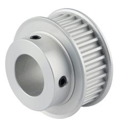
Sung-Il Machinery timing pulley, aluminum, 5mm 5M pitch, 32 tooth, 2.005in pitch diameter, 7/8in bore, hub with flanges. For use with 15mm wide belt.
