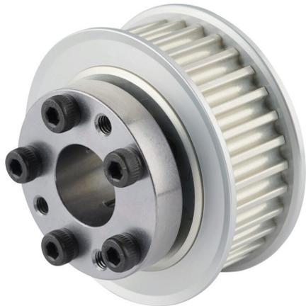
Sung-II Machinery timing pulley, aluminum, 5mm 5M pitch, 32 tooth, 2.005in pitch diameter, 5/8in bore, no hub with flanges. For use with 15mm wide belt. QD bushing included.
