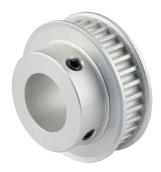
Sung-II Machinery timing pulley, aluminum, 5mm 5M pitch, 32 tooth, 2.005in pitch diameter, 7/8in bore, hub with flanges. For use with 9mm wide belt.
