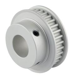
Sung-II Machinery timing pulley, aluminum, 5mm 5M pitch, 32 tooth, 2.005in pitch diameter, 3/4in bore, hub with flanges. For use with 9mm wide belt.
