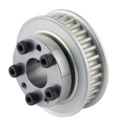
Sung-Il Machinery timing pulley, aluminum, 5mm 5M pitch, 32 tooth, 2.005in pitch diameter, 5/8in bore, no hub with flanges. For use with 9mm wide belt. QD bushing included.
