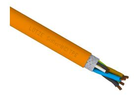
LUTZE Silflex flexible servo cable, shielded, 4 conductors (includes ground), 16 AWG, bare copper, (1) shielded 18 AWG twisted pair, PVC/Nylon conductor insulation material, brown, black, blue and green/yellow ground, TPE jacket, orange, cut to length.
