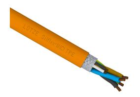
LUTZE Silflex flexible servo cable, shielded, 4 conductors (includes ground), 14 AWG, bare copper, (1) shielded 18 AWG twisted pair, PVC/Nylon conductor insulation material, brown, black, blue and green/yellow ground, TPE jacket, orange, cut to length.
