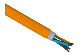
LUTZE Silflex flexible servo cable, shielded, 4 conductors (includes ground), 12 AWG, bare copper, (1) shielded 18 AWG twisted pair, PVC/Nylon conductor insulation material, brown, black, blue and green/yellow ground, TPE jacket, orange, cut to length.
